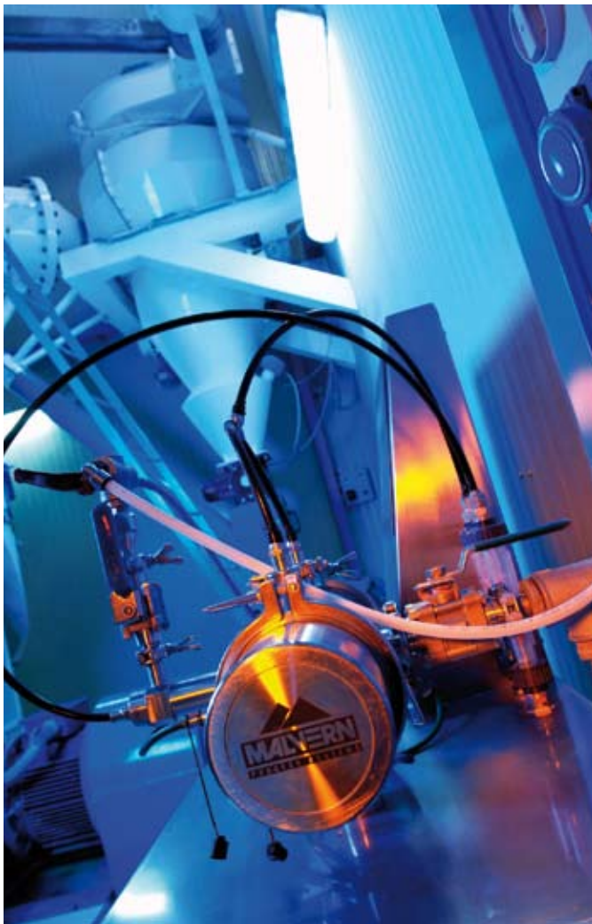
Figure 3: The Insitac, showing connection lines to the process. All pictures courtesy of Malvern Instruments Ltd.
